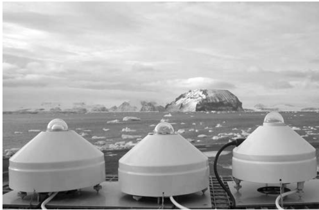
Figure 2. The radiometers equipped with the Kipp & Zonen CV2 ventilation units installed on a special platform at the Mendel Station.
